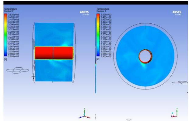
(a). inner wall temperature (coolant temperature) is 80°C
