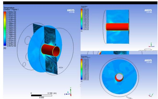
(b). inner wall temperature (coolant temperature) is 90°C
