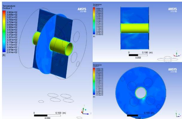
(b). inner wall temperature (coolant temperature) is 90°C
