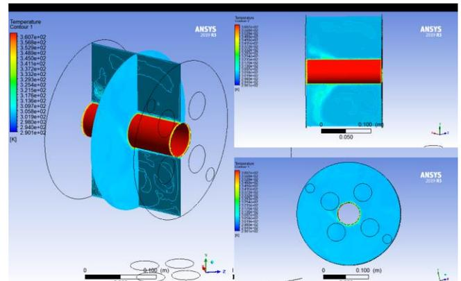
(b). inner wall temperature (coolant temperature) is 90°C
