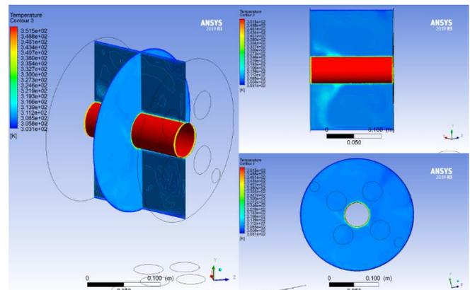
(a). inner wall temperature (coolant temperature) is 80°C
